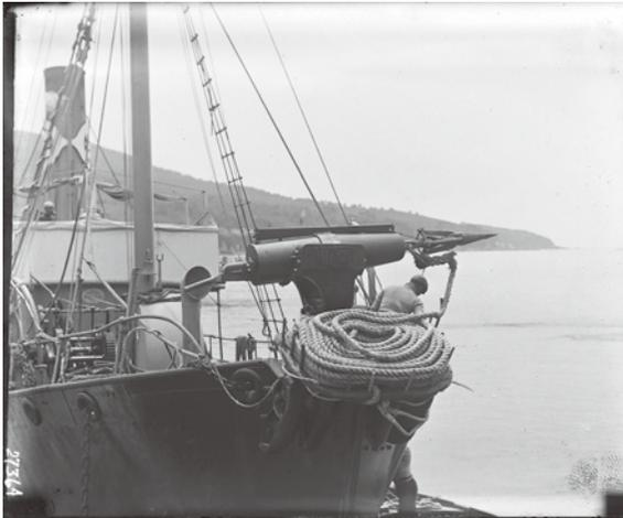
“The harpoon gun on the *Rex Maru*. The gun is loaded and the harpoon is shown projecting from the muzzle ; coiled on the iron pan below is the rope which is carried with the iron in its flight. The winch may be seen in front of the bridge at the left of the picture.”
